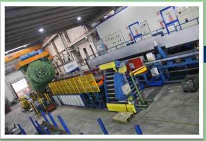
Manipulator system by means of 500 kgs. anthropomorph kuka robots handling the different forging steps. In telematics connection.
