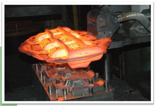
Forging becomes in this way a high industrialized process. Robotization of the line imposes a careful definition and controls of each step of the process.
