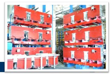
Double system of 3500 KW induction furnaces with temperature control.
