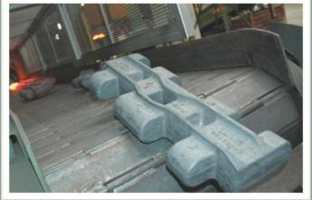
Controlled cooling system to ensure proper structure and surface of forgings.
