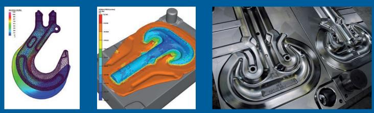
Technicians use modern Computer Aided Design, forging simulation software, and Finite Element Modeling.
